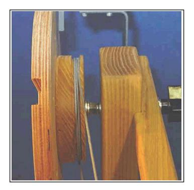
c.) Take the end with the quick link and attach the quick link to the eyebolt under the white cord. Close the threaded side of the quick link.
