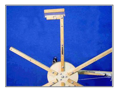
b.) Using the 1/4" x 2-1/4" carriage bolt (hardware #4), attach the raddle mount/adjustable raddle holder assembly to the raddle support. Secure with the flat washer and hex nut.
